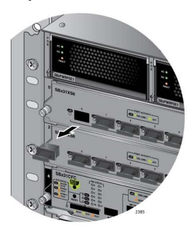
Figure 95. Removing a Dust Cover From an SFP+ Slot in the AT-SBx31XS6 Line Card
